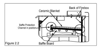
Ceramic Blanket and Baffle Board MUST be in contact with the back of the firebox and even with each other in the front. Baffle Protection Channel MUST be in position.
