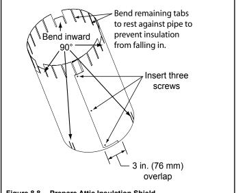
Figure 8.8 Prepare Attic Insulation Shield
