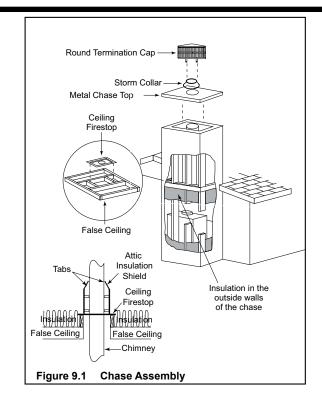
WARNING! Risk of Fire! You must maintain a minimum 2 in. (51 mm) air space clearance to insulation and other materials surrounding the chimney system.
