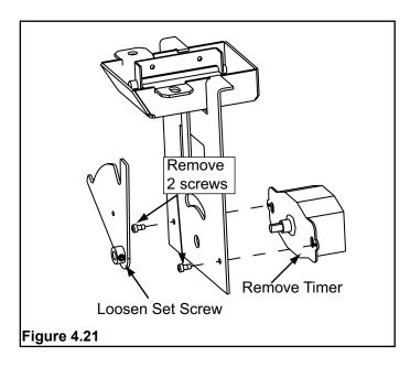
2. Install new timer using same 2 screws. It is very important that the D cut side of the timer shaft is facing the opposite side of the linkage timer arm. Figure 4.22
