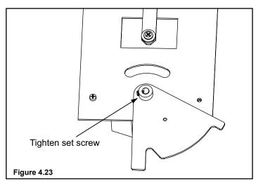
Rotate linkage control arm into final position and reattach to mounting plate. Note that the D cut is now facing the linkage timer arm. Re-attach the linkage timer arm. Figure 4.23.
