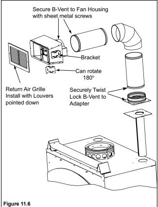
**NOTICE:** Secure the duct so that clearance to the fireplace outer wrap is maintained. <u>Tape all seams with aluminum tape 1-1/4 in. (32mm) minimum width or as specified by local codes.)</u>
