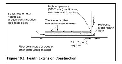
The construction of, and materials used for a hearth extension are shown in Figures 10.1 and 10.3. A hearth extension of this construction may be covered with any non-combustible decorative material and may have a maximum thickness as per Figure 10.2 Seal gaps between the hearth extension and the front of the fireplace with a bead of non-combustible sealant.
