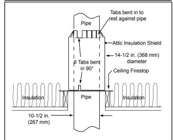
Figure 8.9 Install Attic Insulation Shield (firestop above ceiling)
