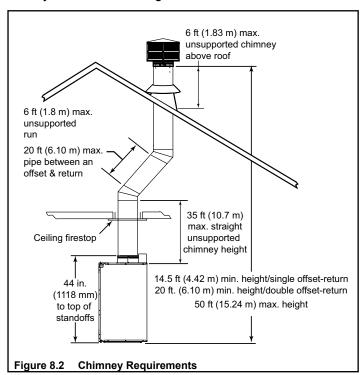
**NOTICE**: You must provide support for the pipe during construction and check to be sure inadvertent loading has not dislodged the chimney section from the fireplace or at any chimney joint.
