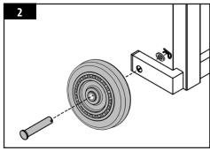
the wheel, then the leg hole, wheel washer, and finally secure using the wheel cotter pin. Note illustration for order. Repeat installation for the other wheel. Once installed, from the rear of the grill, lift the grill into an upright position.
