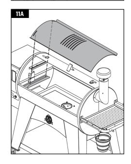
covering the slotted openings. Ensure the raised tab is on the left, to easily adjust for direct or indirect flame when cooking. Note illustration 11B.
