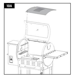
piece to the left side, and the tray will lock into the raised edges above the burn pot. Note illustration 10A. The flame broiler main plate is used to distribute the heat evenly.
