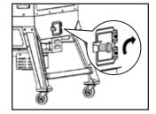
Check and clean off any debris from the fan air intake vent, found on the rear underside of the smoke cabinet. For
