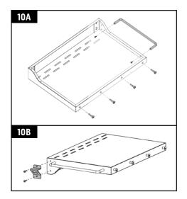
Last, remove the two pre-mounted screws for the bottle opener, and re-install on the corner of the side shelf. Note illustration 10B.
