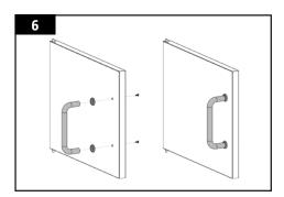
front. Add a cabinet door bezel on the screw, then hand-tighten the screw (from the rear) into the cabinet door handle. Continue to secure the handle by inserting a screw into the other side and tightening.
