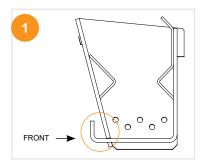
Confirm three baffles inside firebox are secure, placing the side baffles before the center
