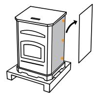
Using a 5/16 inch wrench, on each side of the Stove remove the two bolts.
