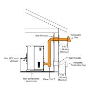
NOTE: In Canada when using a factory-built chimney it must be safety listed, Type UL103 HT (2100<sup>O</sup>F) CLASS "A" or conforming to CAN/ULC-S629M, STANDARD FOR 650°C FACTORY-BUILT CHIMNEYS.
