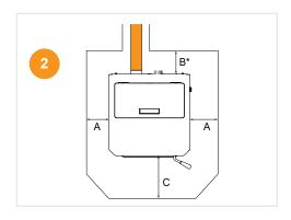
Non-combustible floor protection extending beneath the flue pipe is required with horizontal venting or under the top vent adapter with vertical installation.
