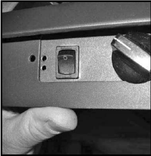
Figure 18: Reinstalling the Speed control assy.
