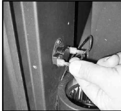
Figure 14: Disconnecting thermal switch.
