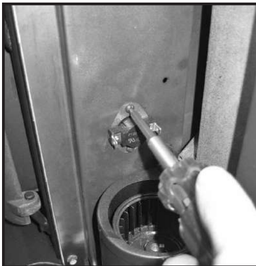
Figure 22: Removing thermal switch.
