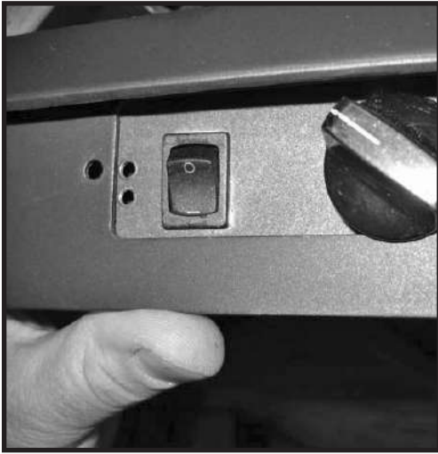
Figure 20: Reinstalling the Speed control assy.
