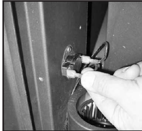
Figure 16: Disconnecting thermal switch.
