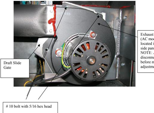
Exhaust Draft Motor (AC model shown) located inside of right side panel NOTE: Always disconnect power before making this adjustment.
