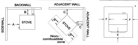
\* Sides of the stove to the front of the grill openings must have a 9"inch clearance.
