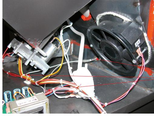
Access to the igniter can be made by opening up the left side panel. The power must be disconnected and make sure that you do not pull on the wiring when taking out the circuit board. The AC model is a little harder to get to than the DC Model that is shown here. Take special care not to cut Yourself or damage wiring.
