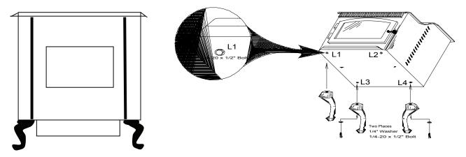
Be careful not to bind the leg when bolting onto the unit so that it does not break. The legs are designed to face at a 45 degree angle so that they will face in the same direction as the slanted side of the face. When the legs are bolted on and positioned where you like them, tighten the (4) four nuts. Make sure not to over tighten the nuts and twist them off.
