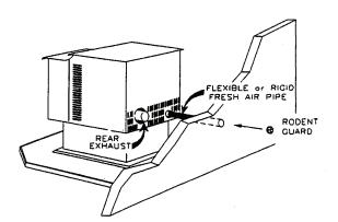
Outside air can be drawn through the floor or through the sidewall.
