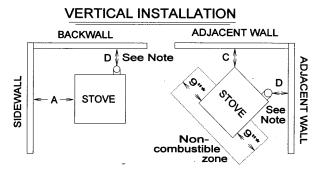
CHIMNEY AND CONNECTOR: 3" LISTED PELLET VENT ONLY NOTE: REGARDLESS OF STOVE CLEARANCE, VENT PIPE MUST ALWAYS HAVE A 3" INCH CLEARANCE.
