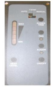
The convection blower speed varies directly with the feed rate. The "Fan" button will override the variable fan function when pressed. It will set the convection blower to high at any feed rate setting.
