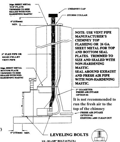
It is best to route the fresh air intake either out the back of the fireplace cavity or down and out to an outside air source. Running the fresh air up and out the top of the chimney can cause excessive draft issues.
