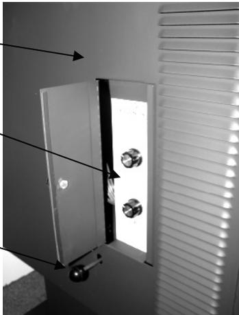
*Pedestal Ash Pan (3500P & 3500L models)* Turn (2) knobs counter clockwise to open ash pan door, pull out ash pan (be sure to wear gloves) and empty into a metal sealed container. Make sure that the ash pan area is clean before putting the ash pan back into place. Close ash pan door and turn knobs clockwise until door is tight and sealed. **NOTE:** the unit will not operate correctly if the door is not closed and latched to get a proper seal.
