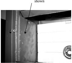
Using the clean-out tool, tap the side heat exchangers that are located on the left and right sides of the firebox. When you open the door, they are located directly inside to the left and right. When you tap the sides with the clean-out tool the loose fly-ash will drop out of these slots.
