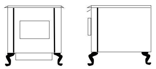
Be careful not to bind the leg when bolting onto the unit so that it does not break. The legs are designed to face at a 45 degree angle so that they will face in the same direction as the slanted side of the face. When the legs are bolted on and positioned where you like them, tighten the (4) four nuts. Make sure not to over tighten the nuts and twist them off.
