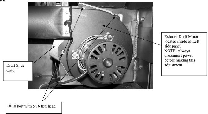
The normal operation of the MagnuM Countryside would be with the Draft Slide Gate open fully as shown. When the gate is in the fully open position, the plate will be against the mounting plate as shown. If the unit needs a draft correction adjustment, the bolts are loosened and the slide gate is rotated a few degrees at a time until the proper operation of the unit is achieved.
