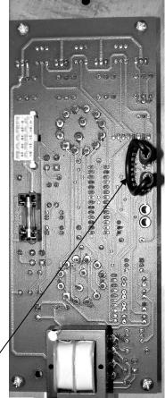
Two (2) <sup>1</sup>/<sub>4</sub>" male spade connectors, one for each wire from wall thermostat
