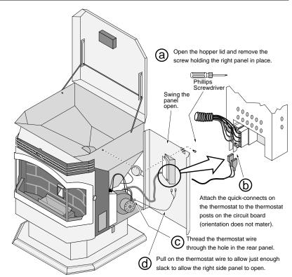
3 Cut the thermostat wire so there is approximately 6" of slack. Expose 1/2" off each wire of the thermostat wire. Attach the exposed wire to the clips on the back of the thermostat using a screwdriver.
