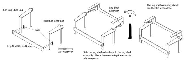
3 Remove the firepot from the pellet stove. Center the log shelf assembly (with extender attached) over the burnpot holder. Replace the burnpot. Place the log on the log shelf extender.
