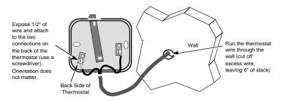
4 Pull the cover off the thermostat. Place the thermostat in location and attach it to the wall through the two obround holes (use the appropriate screws for the type of wall it is being attached to). Replace the cover on the thermostat to complete the installation.
