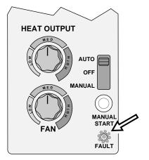
To reset the fault light, turn the mode switch to off and re-start the stove.
