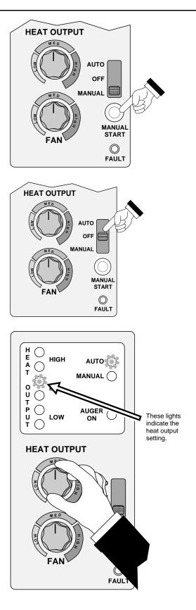
Adjust the "Heat Output" dial to meet the heating requirements you desire.
