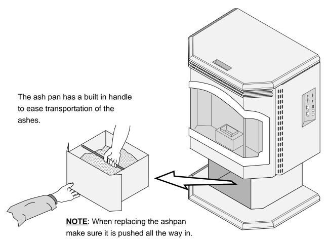
**Disposal of Ashes** – Ashes should be placed in a metal container with a tight fitting lid. The closed container of ashes should be placed on a noncombustible floor or on the ground, well away from all combustible materials, pending final disposal. If the ashes are disposed of by burial in soil or otherwise locally dispersed, they should be retained in the closed container until all cinders have been thoroughly cooled.
