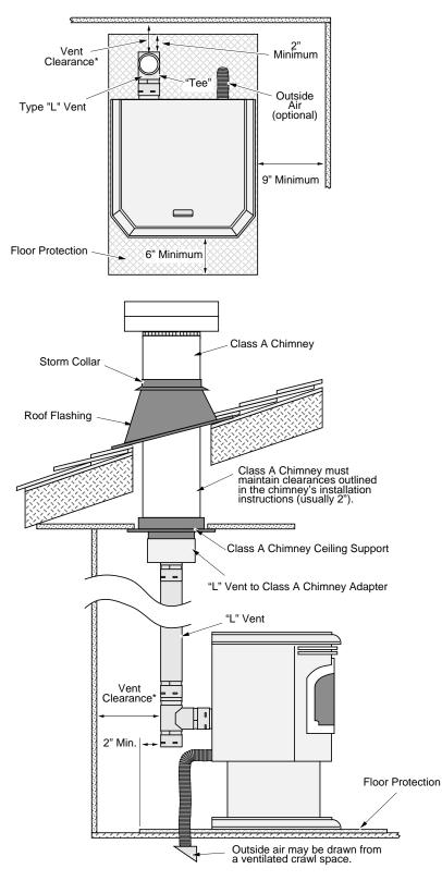
\* Install vent at clearance specified by the vent manufacturer.
