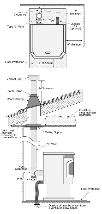
\* Install vent at clearance specified by the vent manufacturer.
