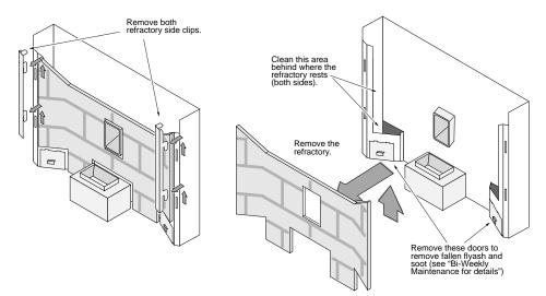
Clean the Exhaust Duct (the stove must be cool and unplugged)
