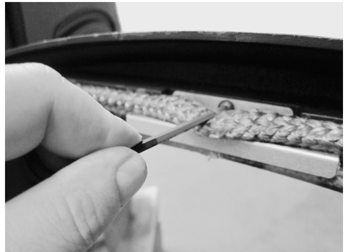
Figure 20. Loosen the glass clips.
