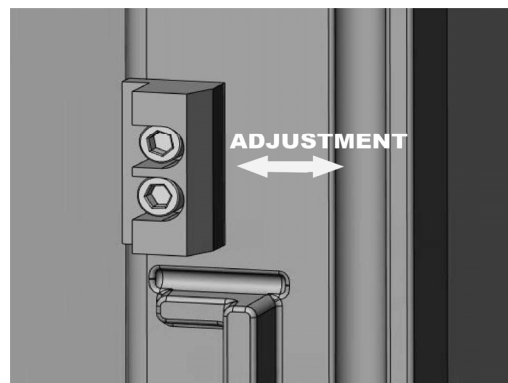
Figure 20: Door Stop Adjustment
