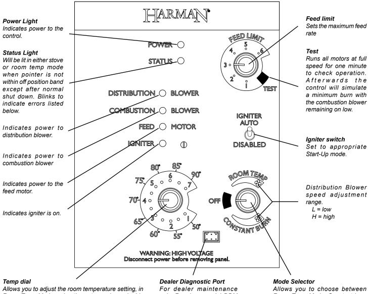
Allows you to adjust the room temperature setting, in Room Temp Mode, using the outer scale marked in degrees Fahrenheit. It also allows you to adjust the constant burn setting, while in Constant burn Mode, using the inner scale marked from 1 to 7.
