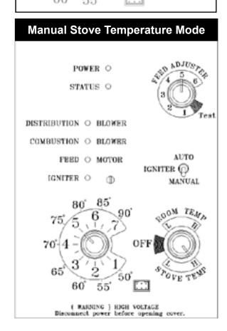
This setting will produce a large viewing fire without a distribution blower operating.
