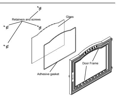
the glass retainers into position and install the screws. Tighten each screw evenly to avoid making any stress points.
