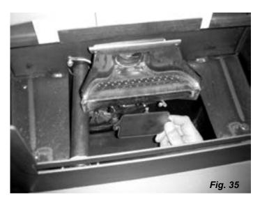
Igniter hot lead wires (high temperature)
