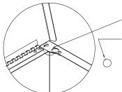
On the rear of the stove hopper there is a hole to fasten the hopper extension into place. On some units, this hole will need to be opened. You will notice a small uncut area on rear of the knockout. Push downward with a screwdriver or like tool until the knockout is rotated as far back to the inside of the hopper as possible. This will allow the swell latch of the hopper extension to fully expand to the bottom side of the hole for a proper seal.
