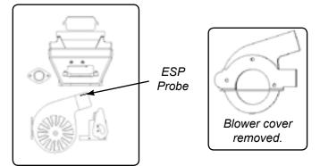
Fig. 30 Exposed blower wheel and flue opening, NOTE: ESP probe is visible.
