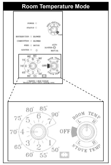
**Room Temperature Mode:** This setting, see above, will produce a room temperature of 70 degrees with the distribution blower at medium speed.
