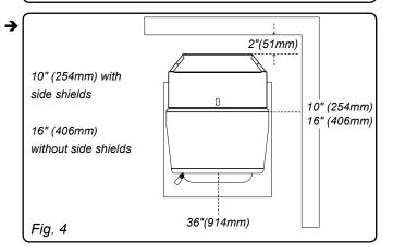
Minimum Size floor protection (USA) is 32<sup>1/2</sup>" wide By 33" deep (825mm X 838mm).
