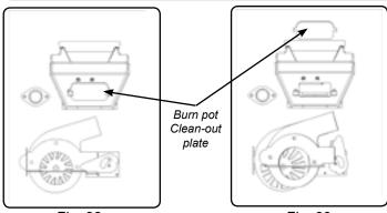
Fig. 28 Latch "closed "with blower cover in place. Burn pot clean-out is closed.
