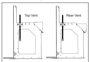
**Note:** When installed in a rear vent configuration, the maximum BTU may be reduced due to elevated ESP temperatures associated with the horizontal exhaust stream.
