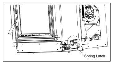
Figure 8.2 - Unlatch spring latch.
