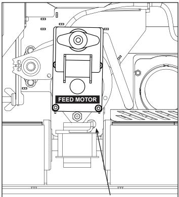
This hole in the feeder body is where the igniter wires pass through to the burn pot.
