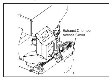
I. Before re-installing the access cover, make sure the insulation between the two layers is in tact.
