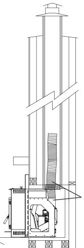
IN CANADA: This fireplace insert must be installed with a continuous chimney liner of a minimum 4" diameter extending from the insert to the top of the chimney. The chimney liner must conform to the Class 3 requirements of CAN/ULC-S635, Standard for Lining Systems for Existing Masonry or Factory Built Chimneys and Vents, or CAN/ULC-S640, Standard for Lining Systems for New Masonry Chimneys.
