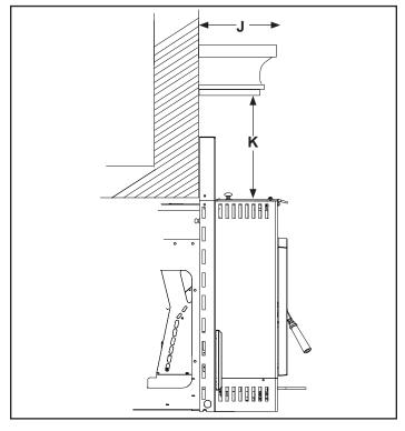
The Maximum mantel depth (J) is 12" (305mm) with a minimum vertical height (K) of 12" (305mm).
