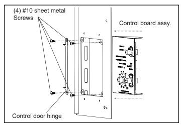
Figure 8.5 - Install control board assembly.
