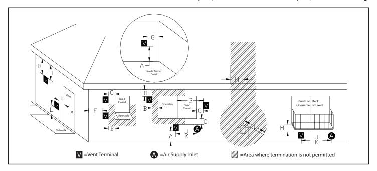
**WARNING:** Venting terminals must not be recessed into a wall or siding.
