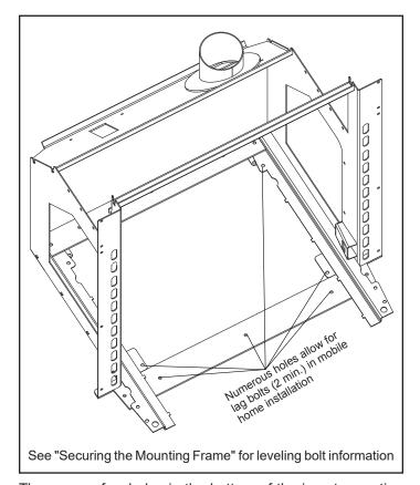
There are a few holes in the bottom of the insert mounting frame which can be used for lag bolts. Use at least two of these holes for securing the appliance to the fireplace floor in a mobile home installation. The installer will need to determine and obtain the properly sized lag bolts and masonry anchors.
