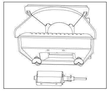
This shows the igniter and bracket removed from the burn pot. Missing in the illustration is the wires from the igniter which run through the burn pot air chamber. Only the first few inches of the wires are insulated for high temperatures. These insulated wires are all that can be inside the feeder or burn pot.
