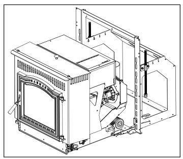
Figure 8.3 - Pull unit away from the mounting frame.
