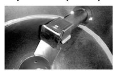
The snap on Pellet Tube Cap is designed to prevent any pellets remaining in the tube from contacting the flame. This is to insure the most efficient combustion; please do not remove the cap.
