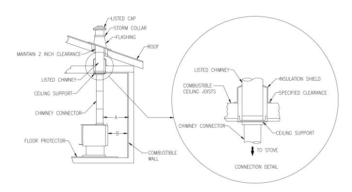
FIGURE 2.2.1 (B) Typical Installation Through the Ceiling
