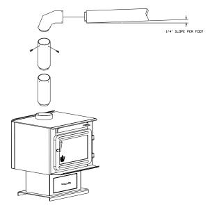
FIGURE 2.3 (B) Minimum Slope
