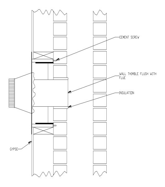
FIGURE 2.2.2 (B) Factory Built Thimble
