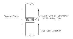
FIGURE 2.3 (A) Connecting Sections
