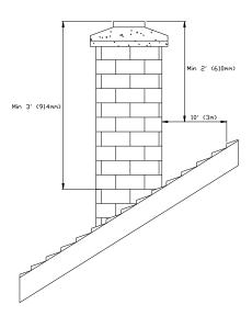
FIGURE 2.2 Minimum Height of the Chimney
