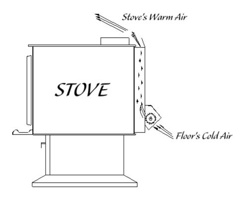
CAUTION: ENSURE THAT THE BLOWER'S POWER CORD IS NOT IN CONTACT WITH ANY SURFACE OF THE STOVE TO PREVENT ELECTRICAL SHOCK OR FIRE DAMAGE. DO NOT RUN THE POWER CORD BENEATH THE STOVE.
