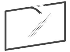
Do not abuse the glass door by striking or slamming shut. Do not use the stove if the glass is broken. To change the glass, perform the same operation described above.
