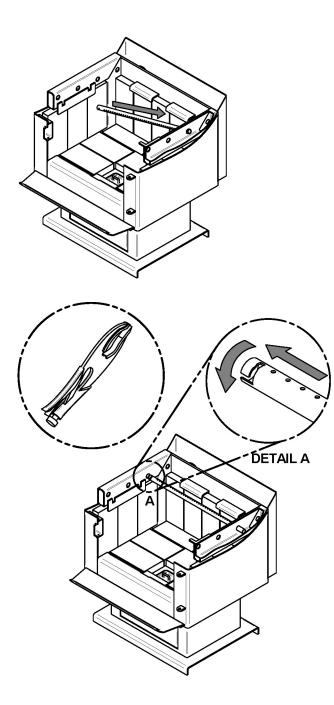
Starting with the rear tube, lean and insert the right end of the secondary air tube into the rear right channel hole. Then lift and insert the left end of the tube into the rear left channel.
