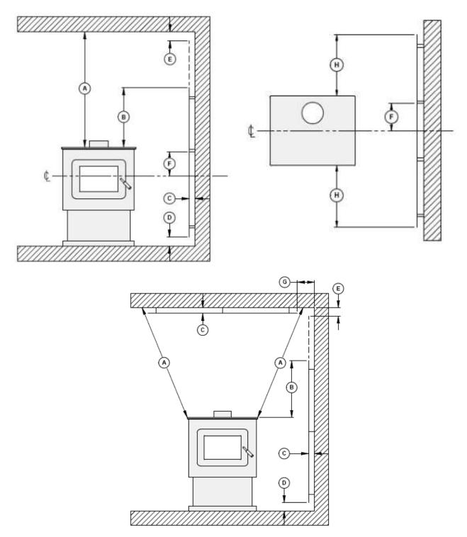
**Clearances for shield construction**
