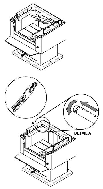
1- Starting with the rear tube, lean and insert the right end of the secondary air tube into the rear right channel hole. Then lift and insert the left end of the tube into the rear left channel.
