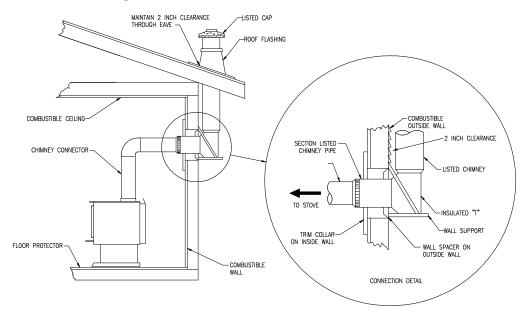
FIGURE 3.2.1 (A) Typical installation through the wall
