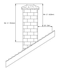
FIGURE 3.2 Minimum Height of the Chimney
