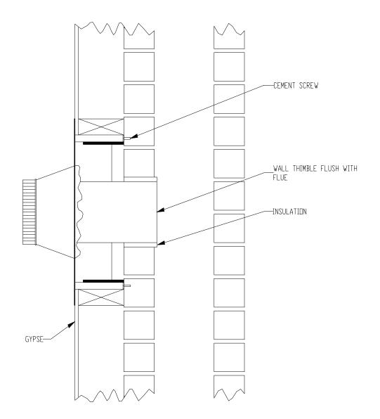
FIGURE 3.2.2 (B) Factory Built Thimble
