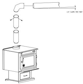
FIGURE 2.3 (B) Minimum Slope
