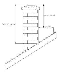
FIGURE 2.2 Minimum Height of the Chimney
