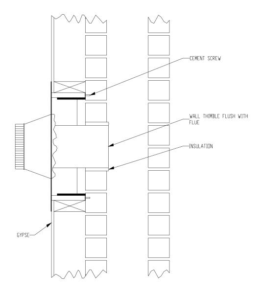
FIGURE 2.2.2 (B) Factory Built Thimble
