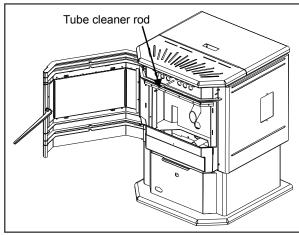
Figure 9: Heat Exchanger Tube Cleaner.
