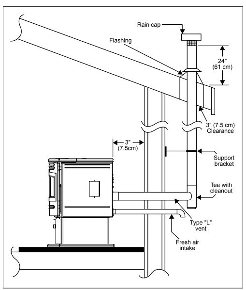
Figure 33: Outside Vertical Installation.
