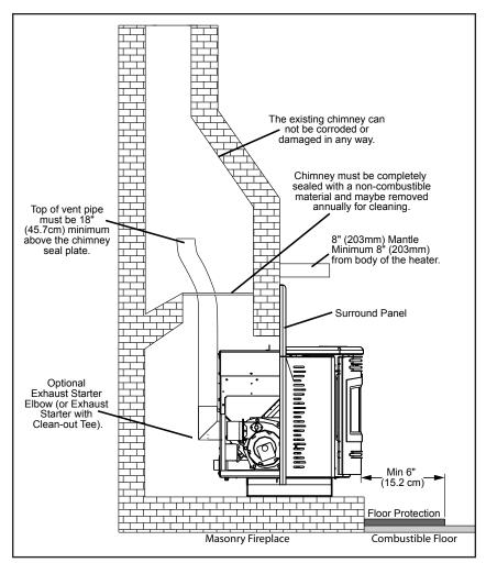
Figure 37: Masonry fireplace positive flue installation.
