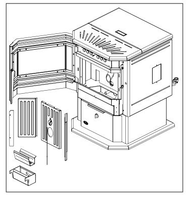
Figure 10: Firebox Components Removal.
