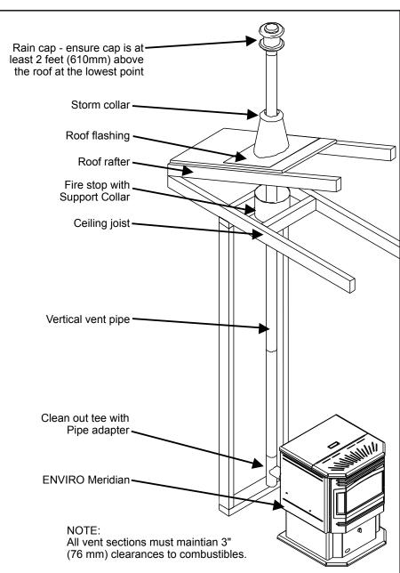
Figure 32: Inside Vertical Installation.
