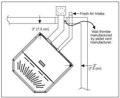
Figure 27: Corner Installation.
