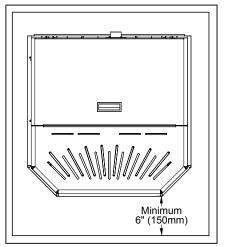
Figure 15: Meridian on Floor Protection.
