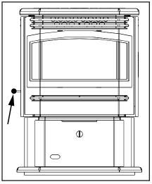
Figure 5: Slider / Damper Knob.
