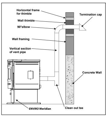
Figure 31: Vertical rise with Horizontal Termination.
