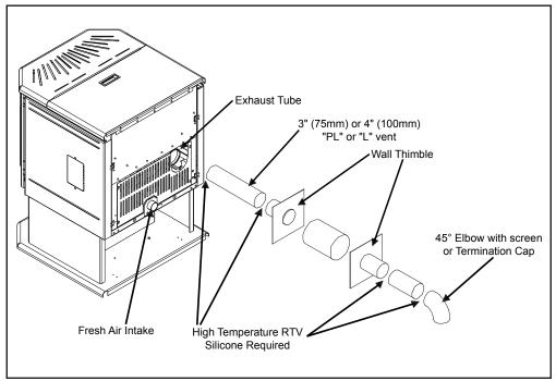
Figure 28: Straight through wall Installation.
