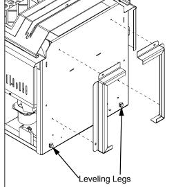
Figure 19: Installing Pedestal.
