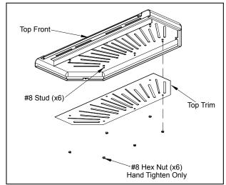
Figure 43: Top front with top tri
