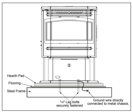
Figure 22: Mobile Home Install Mounting.
