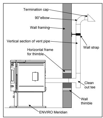
Figure 30: Through Wall with Horizontal Termination.
