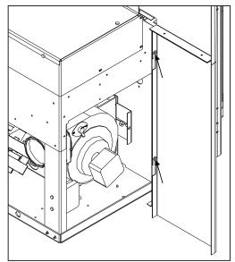
Figure 41: Installed Surround Panel.
