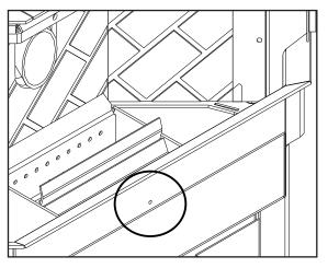
Figure 7: Hole for Pressure test with Magnehelic Gauge.
