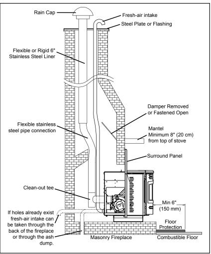
Figure 36: Installation of Fireplace Insert.
