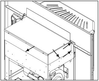
Figure 20: Hopper Cover Screw Placement.
