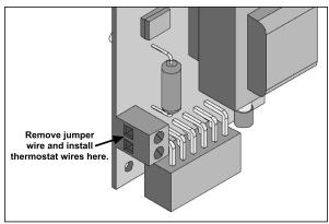
Figure 46: Thermostat wire placement.
