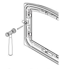
Figure 8: Installing the split pin
