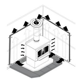
Warning: Note that to reduce the clearances of an appliance using a single wall pipe connector, the use of a heat shield certified with the single wall pipe connector to be used as close as 6" from combustible materials must be used. Only in this case, the same clearances as a certified double wall pipe connector can be used.
