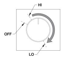
The blower has a variable speed control that can be adjusted in three different positions; either from high (HI) to low (LO) or closed (OFF). Allow the stove to reach operating temperature (approximately one hour) before turning on the blower, since increased airflow from the blower will remove heat and affect the start up combustion efficiency.
