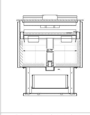
Figure 5: Front View - Combustion Chamber
