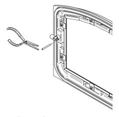
Figure 7: Removing the split pin
