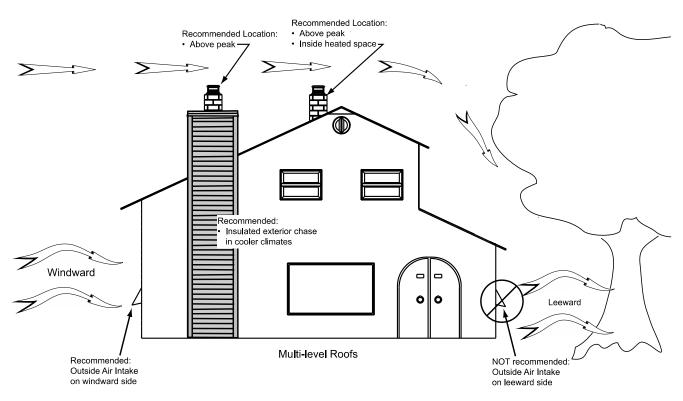
Figure 14: Air supply in conventional houses
