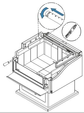
Note that secondary air tubes (A) can be replaced without removing the baffle board (B) and that all tubes are identical.
