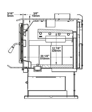
Figure 6: Side View - Combustion Chamber
