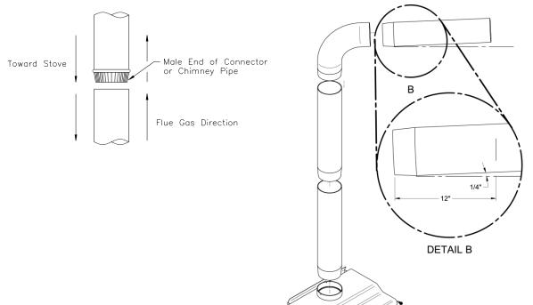
FIGURE 3.3 (A) Connecting Sections
