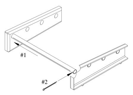
Figure 5.7 – Secondary air tube replacement
