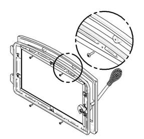
1- Position the overlay on the door frame and fix it in place from behind using the 4 screws.
