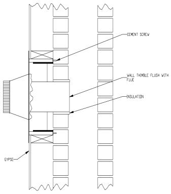
FIGURE 3.2.2 (B) Factory Built Thimble
