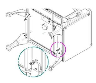
2 (A) - Fix the pedestal base using the 4 bolts and 2 (B) - Fix the 2 legs supports using the 4 bolts washers removed in the previous step.
