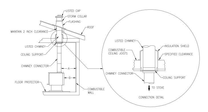
FIGURE 3.2.1 (B) Typical Installation Through the Ceiling
