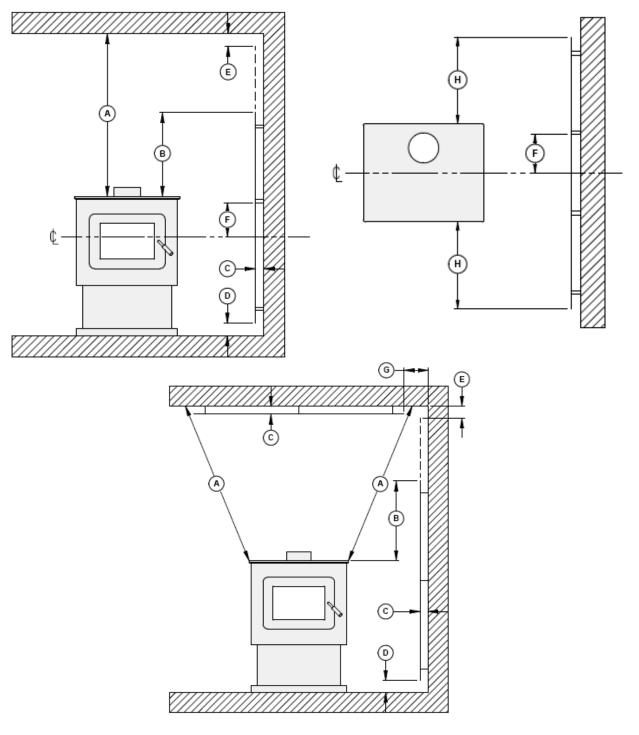
**Clearances for shield construction**
