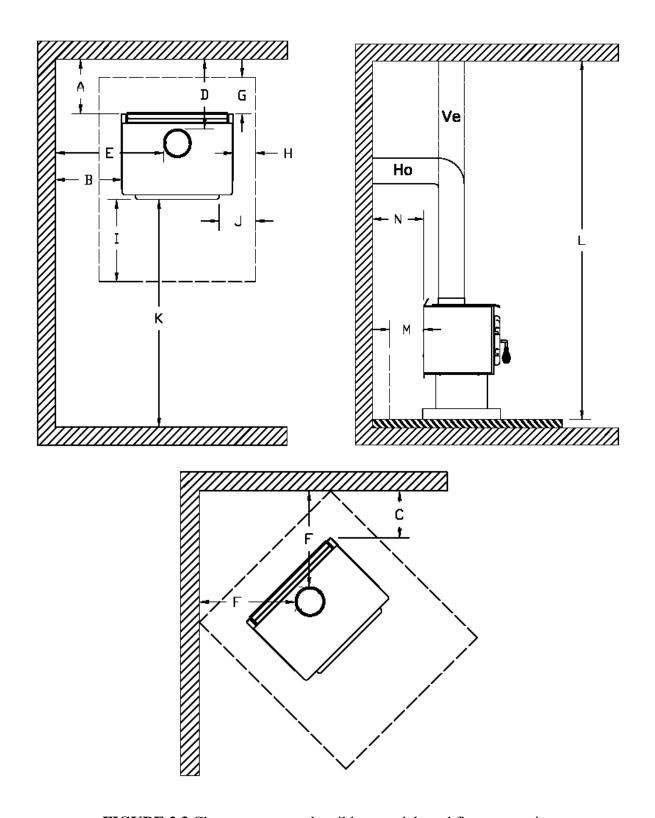
FIGURE 2.3 Clearances to combustible materials and floor protection
