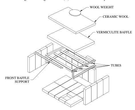
Figure 5.6.2 (A) - Baffle installation
