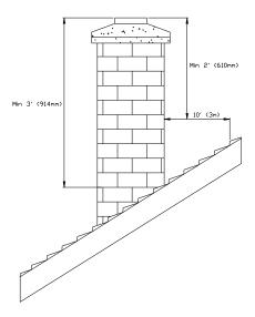
FIGURE 3.2 Minimum Height of the Chimney
