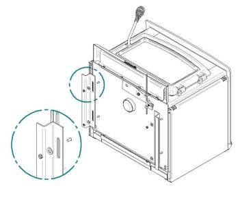
1- Unscrew the 4 bolts in order to remove the 2 steel supports. Dispose of the two steel supports. They are no longer required.
