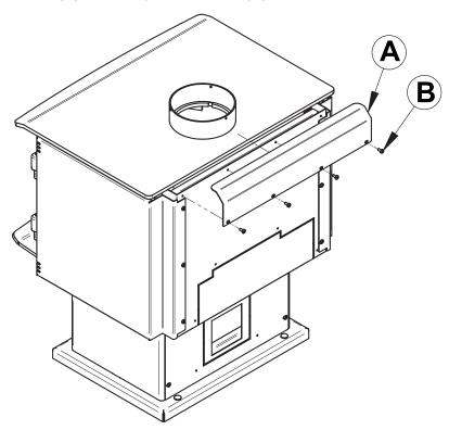
2. Install the airmate (C) with the screws kept from the previous step (B).
