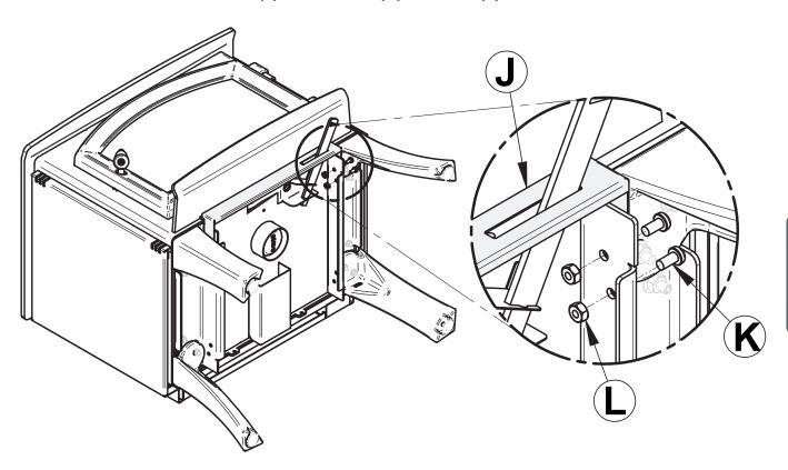
6. Put the stove on its legs, install the ash drawer included with the kit. Put back the firebricks, the ash plug and the door on the stove. See step 1.
