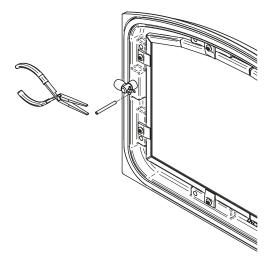
Figure 18: Removing the split pin
