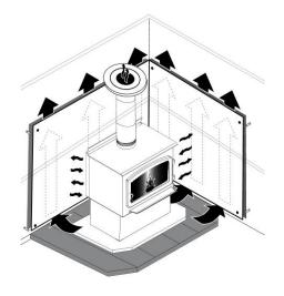
Figure 24: Heat shield
