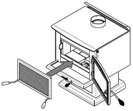
Hold the fire screen by the two handles and bring it close to the door opening.
