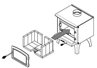
9- Position the stove for its installation and reinstall the bricks, ash plug and loading door (see Appendix 9: Exploded Diagram and Parts List for bricks layout).
