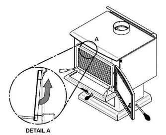
Lean the upper part of the fire screen against the top door opening making sure to insert the top fire screen brackets behind the primary air deflector as in (Detail A).
