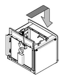
3- Remove the (2) transport support bracket (A) which can be discarded. Keep the (4) bolts (B), washers (C) and nuts (D) since they will be required in **step 5**.
