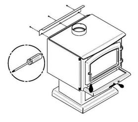
5- Slide the panels into the front brackets and reinstall the panels and top air deflector using the screws removed in **step 1**.
