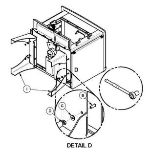
4- Secure both leg support assembly (I) (to the underside of the firebox using the bolts, washers and nuts removed in **step 3**. Supports can be installed on either side.
