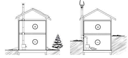
Good System Design Inside chimneys are preferred because even when no fire is burning, there is normally upward flow in the system.
