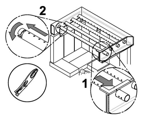
Starting with the rear tube, lean and insert the right end of the secondary air tube into the rear right channel hole (**DETAIL 1**). Then lift and insert the left end of the tube into the rear left channel.
