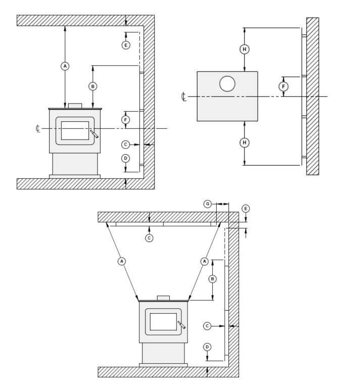
**Clearances for shield construction**
