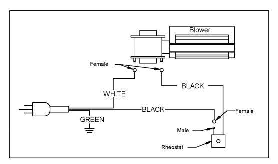
CAUTION: ENSURE THAT THE BLOWER'S AND/OR THE THERMODISC'S POWER CORD ARE NOT IN CONTACT WITH ANY SURFACE OF THE STOVE TO PREVENT ELECTRICAL SHOCK OR FIRE DAMAGE. DO NOT RUN THE POWER CORD BENEATH THE STOVE.
