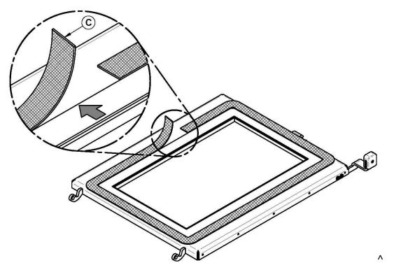
Apply self-adhesive gasket (C) en following the engraving on the inside of the door frame.
