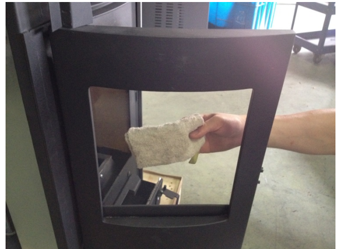
Figure 31: Wipe glass and inspect gasket
