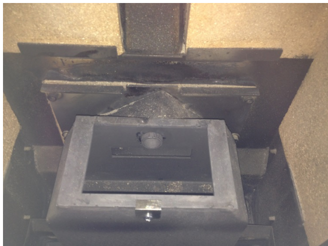
Figure 35: Remove ash from ignitor tube (underneath repot)
