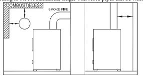
9" of combustibles provided an approved fire retardant material covered with 28 gauge sheet metal, spaced out 1" on non-combustible spacers, is utilized. See illustration.
