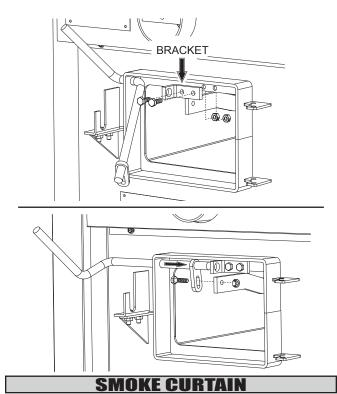
Using two  $1/4-20 \times 1-1/4$ " Carriage bolts, the smoke curtain clips and two nuts, attach the smoke curtain in place above the Fuel Feed Door as shown below. After installation, the smoke curtain should swing freely back into the furnace.
