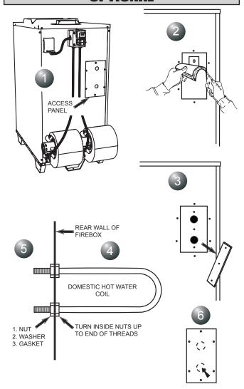
This Furnace will accept the installation of a Domestic Hot Water Coil Kit. The kit is a 1124 Water Coil and it may be purchased from your local dealer.
