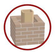
This appliance must be connected to a listed high temperature (ULC629 IN CANADA OR UL-103HT IN THE USA) residential type factory build solid fuel chimney or an approved masonry chimney with a flue liner.
