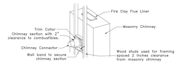
Fig. 16 Metal Prefabricated Thimble
