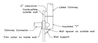
Fig. 18 Detail Of Connection Through Wall
