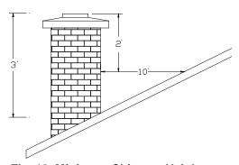
Fig. 12 Minimum Chimney Height
