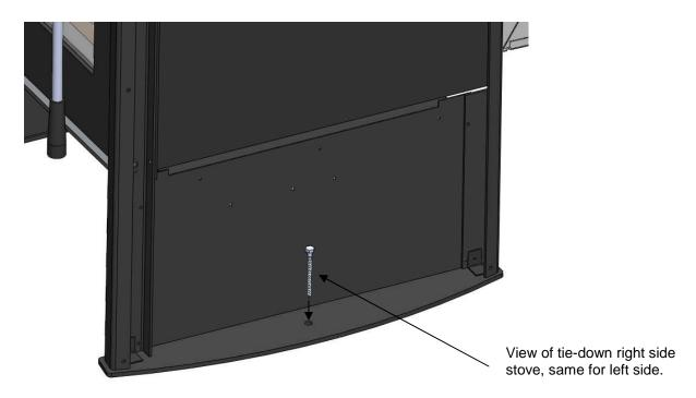
In mobile home installations, the stove must be securely fastened to the floor using the tie-downs provided in the Outside Air kit. (To access the screw down hole, remove side shields (see page 23)).
