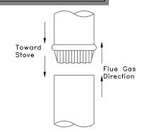
Fig.8 Flue Gas Direction
