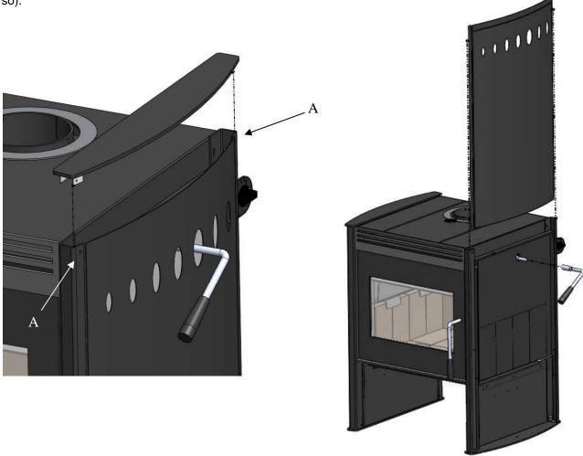
If you like to install the flat versus the curved shields or vise versa, the matching cover plate on the bottom need to be replaced too. This can be done by undoing the two screws (B) holding the bottom plate in place. An extra person or jack might be required to lift the one side of the stove. Check stove pipe and possible fresh air connection before doing so. If installed in mobile home, remove floor anchor prior to lifting stove.
