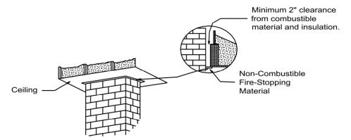
Fig. 11 Clearances—Masonry To Combustibles
