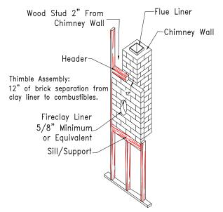
Fig. 13 Brick Chimney Thimble
