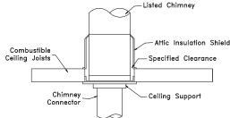
Fig. 17 Detail Of Connection Through Roof
