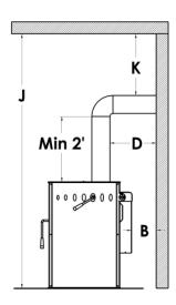
G = 4" in USA 8" in Canada H = 16" in USA 18" in Canada I = 0" in USA 8" in Canada K = 18" for single wall pipe in Canada (If K=18", J=84" Minimum)
