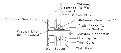
If an exterior masonry chimney is used you may have draft problems due to the chimney being too cold. Exterior masonry chimney's should be lined with a listed (insulated) stainless steel liner for better operation of these units.
