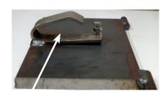
APPLY LUBE TO THE UNDER SIDE OF THE BYPASS RAMP
