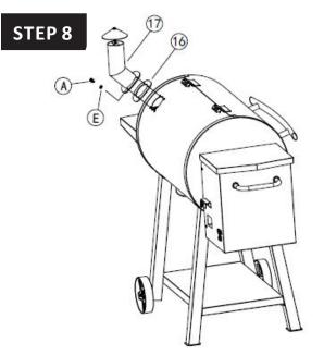
Assemble the stack (17) and gasket (16) to the main body with 4 bolts (A) and 4 washers (E).
