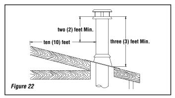
**Note:** 2" clearance to combustibles around chimney components required.
