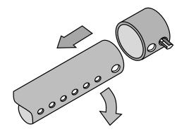
**b** Slide the air tube to the left, swing it down and remove from the firebox.
