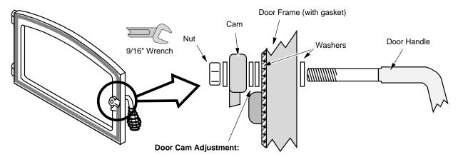
To tighten the door cam, remove the door handle and discard one of the washers between the door frame and cam. To loosen the door cam, add a washer between the door frame and cam.
