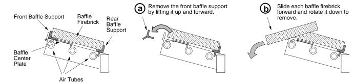
The baffle center plate rests on the side air channels. Its back edge (the larger flange) rests against the center air tube. Remove it by sliding it forward and out.
