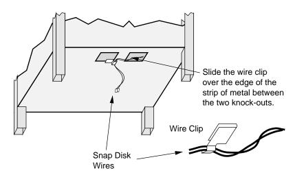
Feed the two snap disk wires into the eye of the wire clip. Remove all slack from the wire, making sure not to dislodge the snap disk. Pinch the eye of the wire clip to secure the wires.
