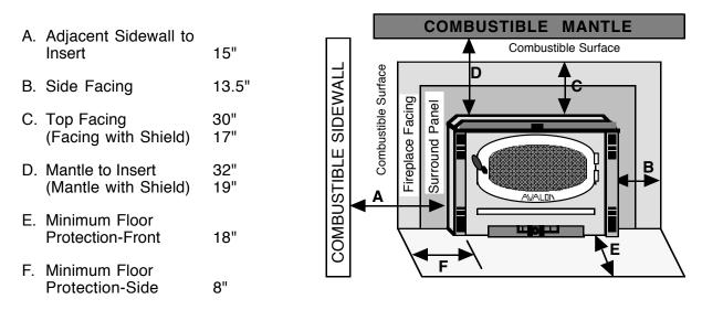
NOTE: For clearances, use this clearance diagram or the clearance diagram on the safety label attached to the back of the appliance.
