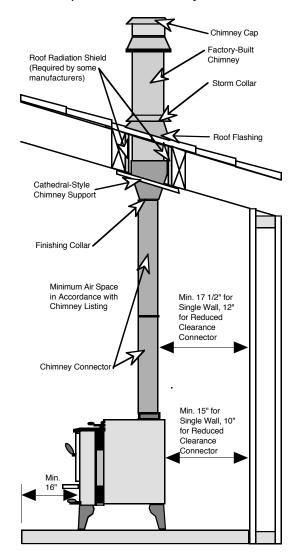
IMPORTANT: Because of the slope of the cathedral ceiling, care should be taken to extend the chimney sufficiently far into the room so that the chimney connector will meet the minimum clearances requirement from the sloped combustible ceiling. The greater the pitch of the ceiling, the further into the room the chimney section must extend. Use the concepts from "CHIMNEY INFORMATION & REGULATIONS" to accurately measure the appropriate distance from a sloping ceiling.
