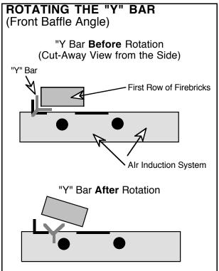
REPLACING THE BAFFLE (TOP) FIREBRICKS & COMPONENTS
