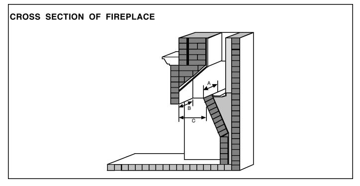
Your template should resemble the drawing on the next page with the dotted lines indicating your initial measurements and the solid line indicating the additional 2". You will use this template to cut a piece of sheet metal (minimum 24 gauge) to install in your smoke chamber.
