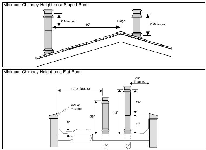
These minimum chimney heights are required by building codes for safety purposes, to allow time for sparks exiting a chimney to cool before they land on the roof. In some problematic situations, additional chimney height above the specified minimums may be necessary to reduce wind-induced down drafting and back puffing, or to increase draft, thereby improving appliance operating characteristics.
