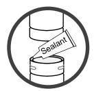
The exhaust system must be completely airtight and properly installed. The pellet vent joints must be sealed with RTV 500° F. (260° C.) silicone sealant.
