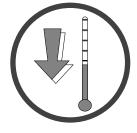
Allow the heater to cool before carrying out any maintenance or cleaning. Ashes must be disposed in a metal container with a tight lid and placed on a non-combustible surface well away from the home or structure.
