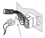
Attach the quick-connects to the two posts near the molex connector on the circuit board (orientation does not mater).
