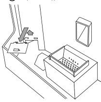
Slide the ash pan trap door forward to expose the ash dumps.
