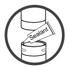
The exhaust system must be completely airtight and properly installed. The pellet vent joints must be sealed with RTV 500° F. (260° C.) silicone sealant.
