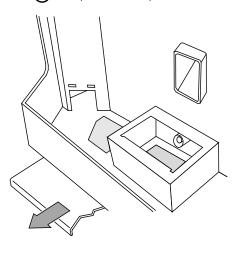
f Replace the ash trap doors and firepot. Slide the ash pan trap door forward.
