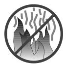
Do not operate the heater if the flame becomes dark & sooty of if the firepot overfills with pellets. Turn the MODE SWITCH to "OFF" and periodically inspect the heater (see "Running Your Heater").
