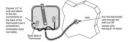
4 Pull the cover off the thermostat. Place the thermostat in location and attach it to the wall through the two obround holes (use the appropriate screws for the type of wall it is being attached to). Replace the cover on the thermostat to complete the installation.
