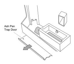
Replace the ash trap doors and firepot. Slide the ash pan trap door forward.
