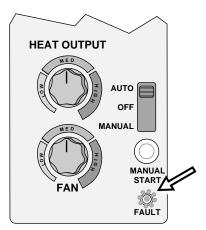
To reset the fault light, turn the mode switch to off and re-start the stove.
