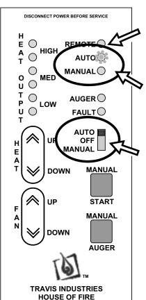
**NOTE**: if using a modulating remote, this light will come on to indicate the remote is controlling the heater.
