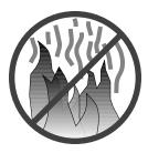
Do not operate the heater if the flame becomes dark & sooty of if the firepot overfills with pellets. Turn the MODE SWITCH to "OFF" and and monitor the heater (see the "Maintenance" section for details).
