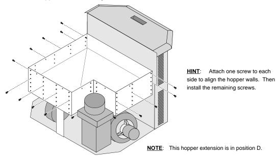
Attach the hopper top following the directions below.
