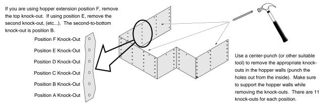
Re-install the hopper walls following the directions below.
