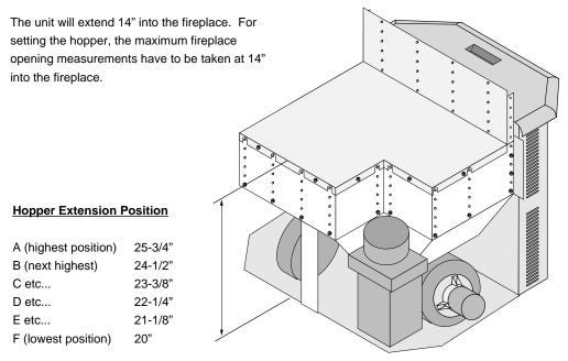
Remove the hopper top following the directions below.
