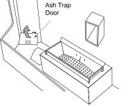
Slide the ash pan trap door forward to expose the ash dumps (the door can be removed and cleaned if necessary)
