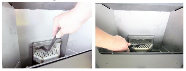
4. Brush away flyash around the fire platform using the brush included with the insert. The flyash will fall into the ashpan below.
