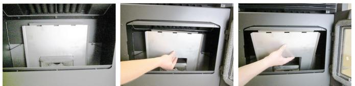
5. With the liners removed, clean all flyash and debris from the firebox. Clean the liners before replacing.
