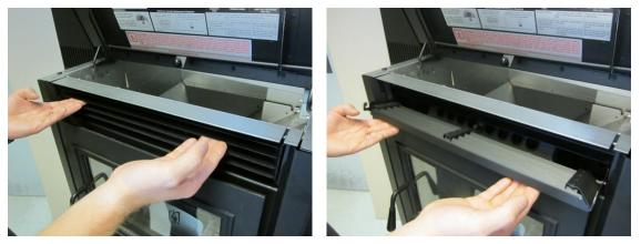
2. Hook the cleaning tool onto the heat exchange scraper rod as shown below.
