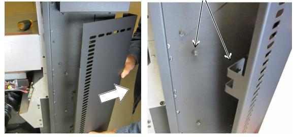
**NOTE**: When re-installing the side panel, make sure the tabs on the panel insert into the slots on the front of the insert
