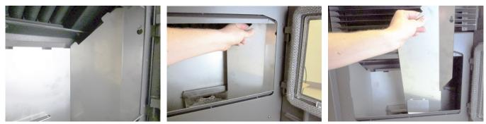
4. Remove the rear liner. Lift it up and remove it from the firebox.
