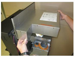
3 Use a center-punch to remove the appropriate knock-outs from the hopper walls (9 total). The holes are punched out from the inside. Make sure to support the hopper walls while removing the knock-outs. In the example below the "A" position is used (tallest hopper position).
