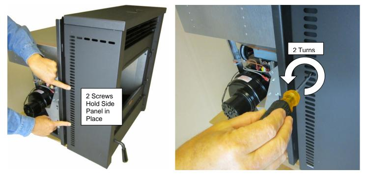
4. Slide each side panel forward and place aside. The side panels have slots that fit over the screws.
