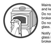
Maintain the door and glass seal and keep them in good condition. Do not operate this heater with broken or missing glass. Do not slam the door or strike the
