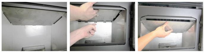
3. Remove the side liners. They have keyhole slots that fit over screws on the side of the firebox. Lift them up, tilt them inwards, then remove.
