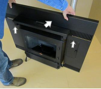
7. The panel has hooks on the sides that fit over slots on the insert. Grasp the panels with both hands, lift slightly, then push forward until all four hooks (and tabs on top of insert) engage the slots on the insert. Double-check panel alignment to verify all hooks have engaged.
