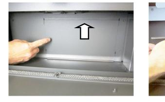
3. Remove the exhaust channel cover plate and gasket (11/32" nutdriver).
