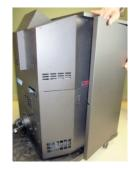
2. Remove the top and bottom screws securing the convection blower cover and remove the cover as shown below (5/16" nutdriver).
