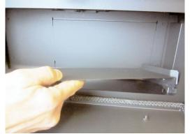
2. Remove the exhaust duct cover as shown below. Press up on it and lift it out.
