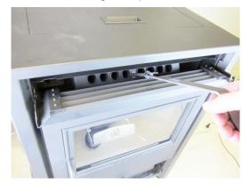
3. Move the scraper rod back and forth a few times to clean the heat exchange tubes.
