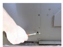
3. Remove the 2 nuts securing the blower using a 7/16" nutdriver. Lift out and remove the convection blower from the stove as shown below.
