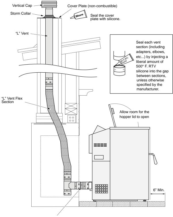
NOTE: you may need a short horizontal section here to clear the lintel and allow the hopper lid to open.
