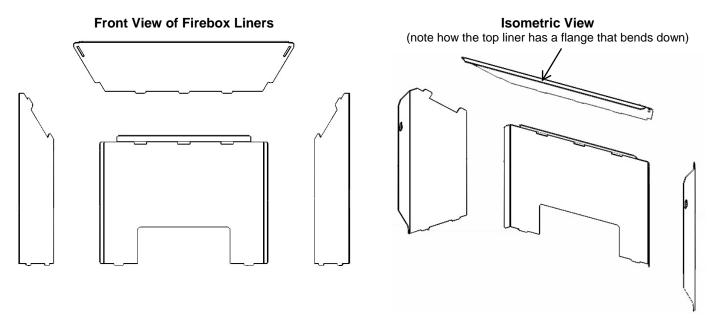
The firebox liners help trap flyash before it enters the exhaust blower. Remove the liners and clean the area behind them following the directions below.
