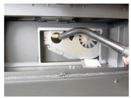
Clean the combustion blower with the bottle brush or vacuum.
