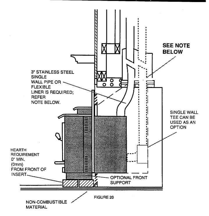
NOTE: A 3" stainless steel single wall pipe or a flexible liner is required to extend to the top of the existing chimney for metal (Z.C.) fireplaces. The existing chimney should be sealed at the bottom or the top with a sheet metal plate or other non-combustible material (i.e. Kaowool or high-temperature fiberglass insulation).
