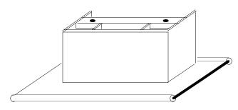
Using a 9/16" open-end or socket wrench, fasten the pedestal to the stove with the supplied bolts and washers. NOTE: Keep the two front leg bolts in place when installing on a pedestal -- otherwise air will enter through these holes.
