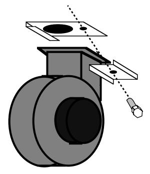
Once the convection fan is removed, place it so the impeller blades are facing up. Check the impeller blades for any damage and replace if necessary. Use a vacuum cleaner or brush to clean away any flyash that may have accumulated. Lubricate the convection fan bearings by dropping two drops of light machine oil into the two holes located on the outward side. Over-oiling can damage your fan.
