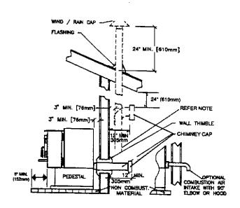
INSIDE VERTICAL INSTALLATION WITH ROOF TERMINATION
