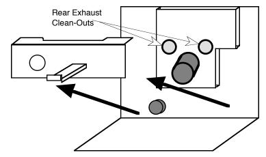
Then brush away any flyash that may have accumulated on the floor of the firebox or on the exhaust ducts with a brush. Then vacuum or dump the flyash into a suitable disposal container.
