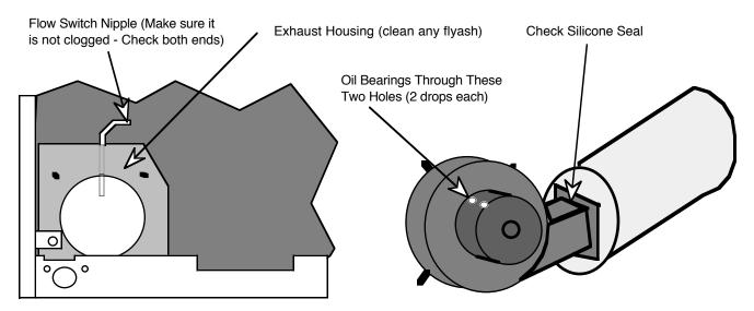
Prior to replacing the fan assembly, check that the silicone seal at the fan and exhaust tube. If fractured, use Type RTV 500 degree silicone sealant to reseal the joint.
